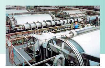
The drum vacuum filters are designed for filtration of difficult to filtrate suspensions in titanium dioxide production (BBM45-3.14-1G), of sodium bicarbonate suspension in soda ash production (BB-5.4 and BYaN-180) as well as in other chemical productions.
