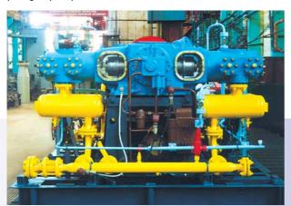
The cylinders are forced cooled by fluid through closed loop.
